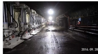
b. Entry formation (Before withdraw support)
