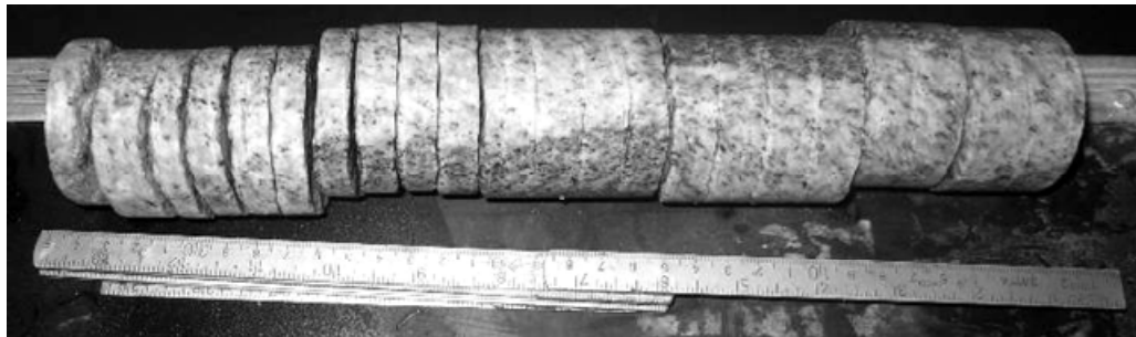
Figure 11. Illustration of core dinking: 23 disks observed in a 27 cm long core.
