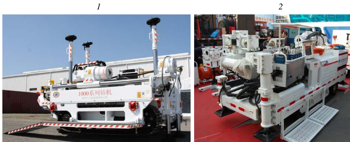
Fig. 1. Directional in-seam drill rigs: 1 – VLD 1000A (Australia), 2 – ZDY 4000 LD (China).
