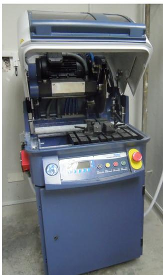
Fig. 1. Circular cutting saw
