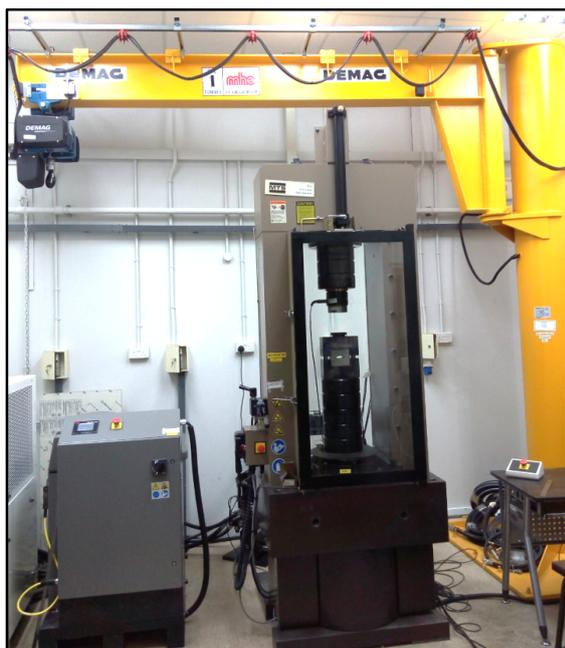
Fig. 13. MTS uniaxial loading frame
