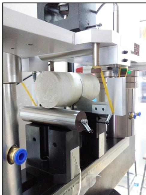
Fig. 14. Conducting a mode-I fracture toughness test
