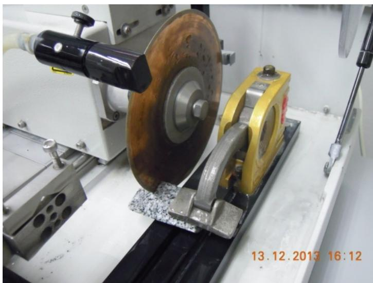
Fig. 2. Linear precision cutting saw
