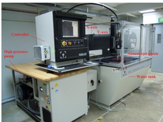
Fig. 5. OMAX 2626 Precision JetMachining Center
