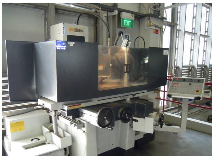
Fig. 3. Automatic surface grinding machine
