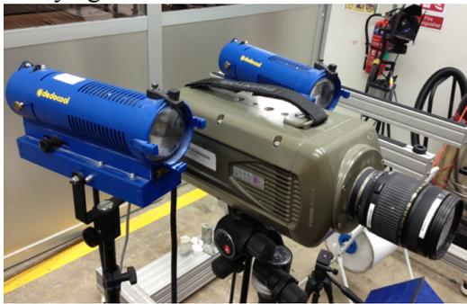
Fig. 8. High speed camera
