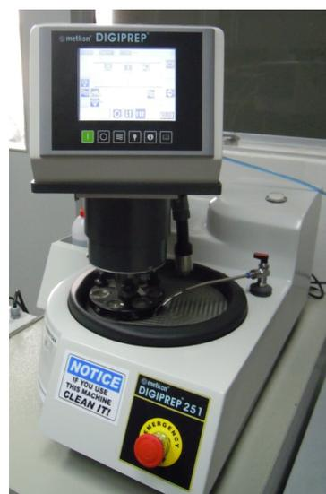
Fig. 4. Automatic sample grinding and polishing system
