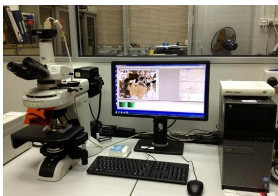
Fig. 6b. Petrographical polarizing microscope
