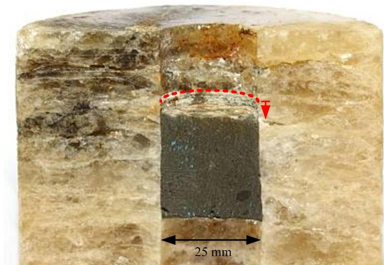
Fig. 6. A cut section of specimen no.SBIIH-04-07-PO-01 after failure in the push-out test.
