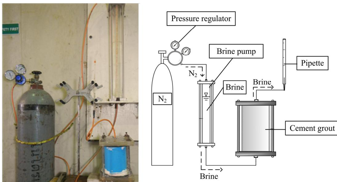
Fig. 10. Constant head flow test apparatus used for the permeability testing of a cement grout.
