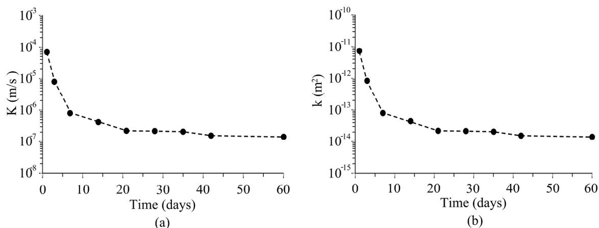
Fig. 11. (a) Conductivity of permeability ( $K$ ) and (b) Intrinsic permeability ( $k$ ) of the cement grouts.
