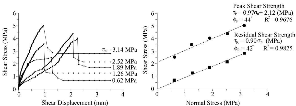
Fig. 8. Results of the direct shear testing.
