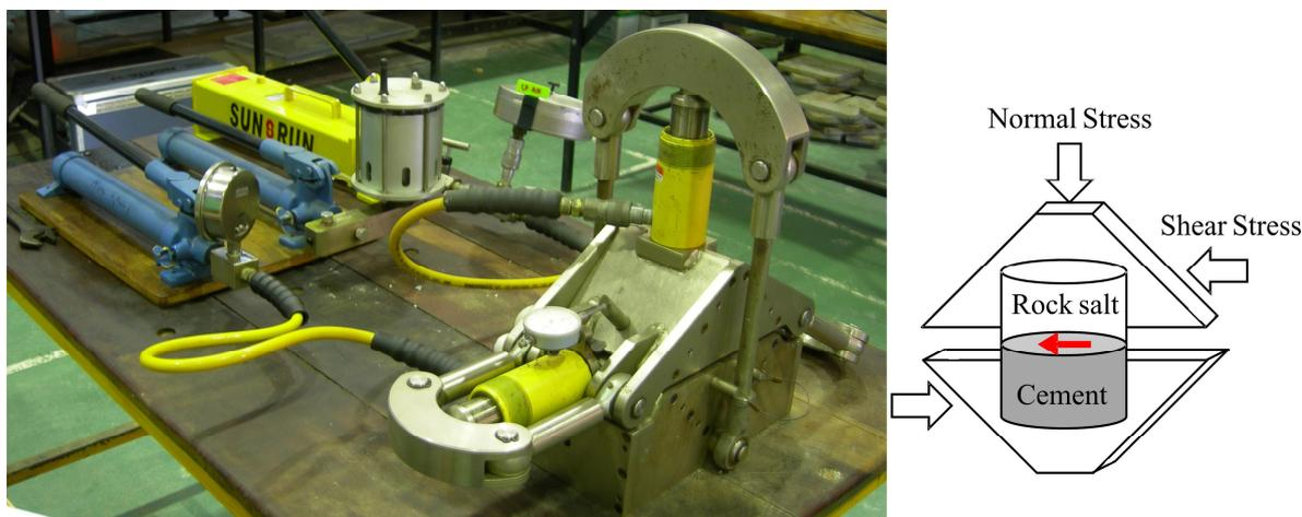
Fig. 7. Laboratory equipment and instrumentation setup for the direct shear test.
