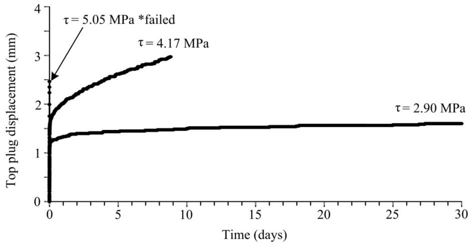
Fig. 5. The top plug displacement as a function of time for the push-out tests.
