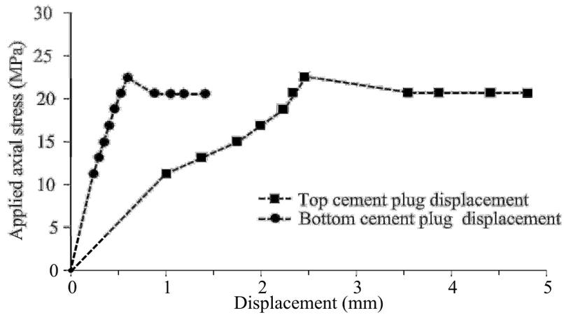
Fig. 4. The applied axial stress as a function of the top and the bottom axial cement plug displacements for the push-out test (specimen no.SBIIH-04-07-PO-01).
