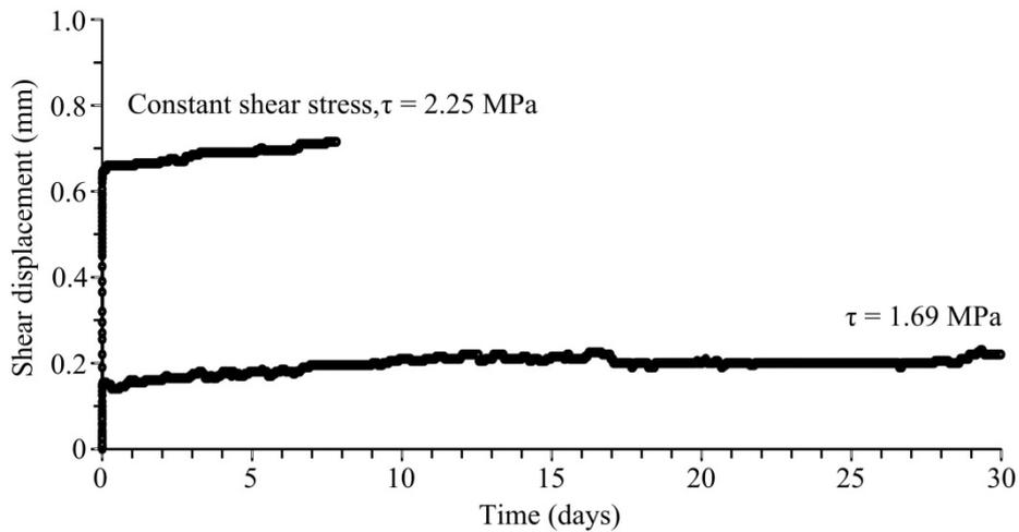
Fig. 9. Shear displacement as a function of time for the direct shear tests with a constant normal stress of 1.86 MPa.
