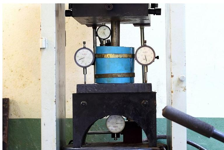
Fig. 3. The push-out test setup.
