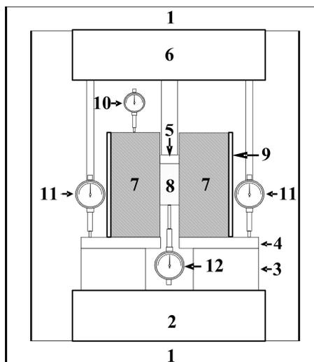
Fig. 2. Schematic drawing of the push-out test setup 1. Loading frame; 2. Hydraulic cylinder; 3. Steel plate with a slit; 4. Square steel plate; 5. Axial bar and steel cylinder; 6. Square steel plate frame; 7. Rock salt sample; 8. Cement grout plug; 9. PVC mold; 10., 11. and 12. Dial gages.
