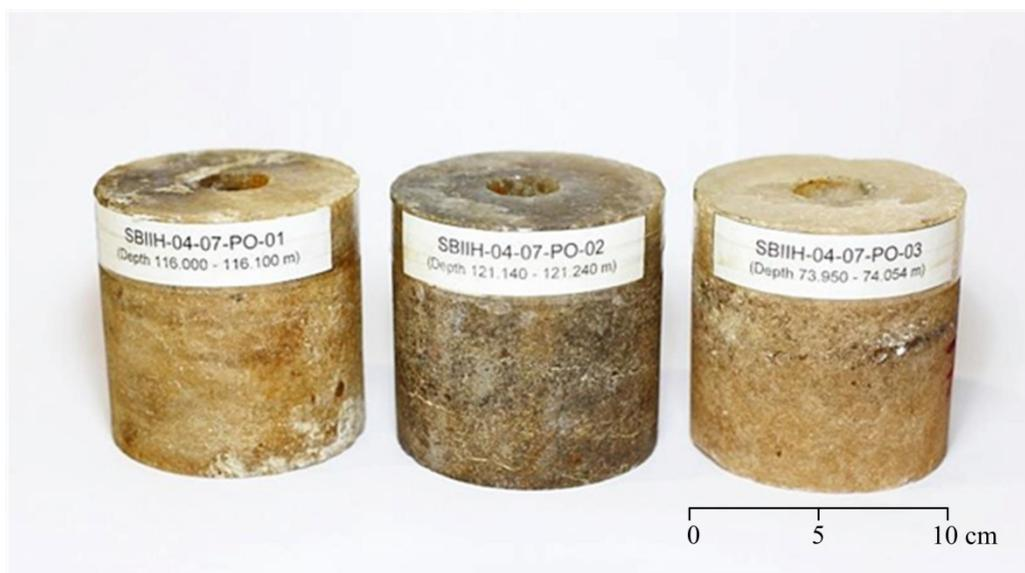
Fig. 1. Examples of salt specimens prepared for push-out test.
