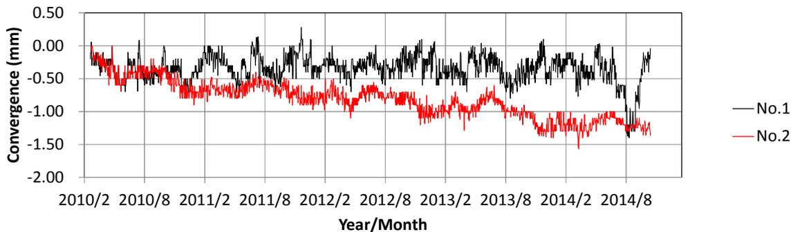
Fig.3. Convergence at No.1 and No.2 unit sections (Negative values correspond to narrowed sections.)
