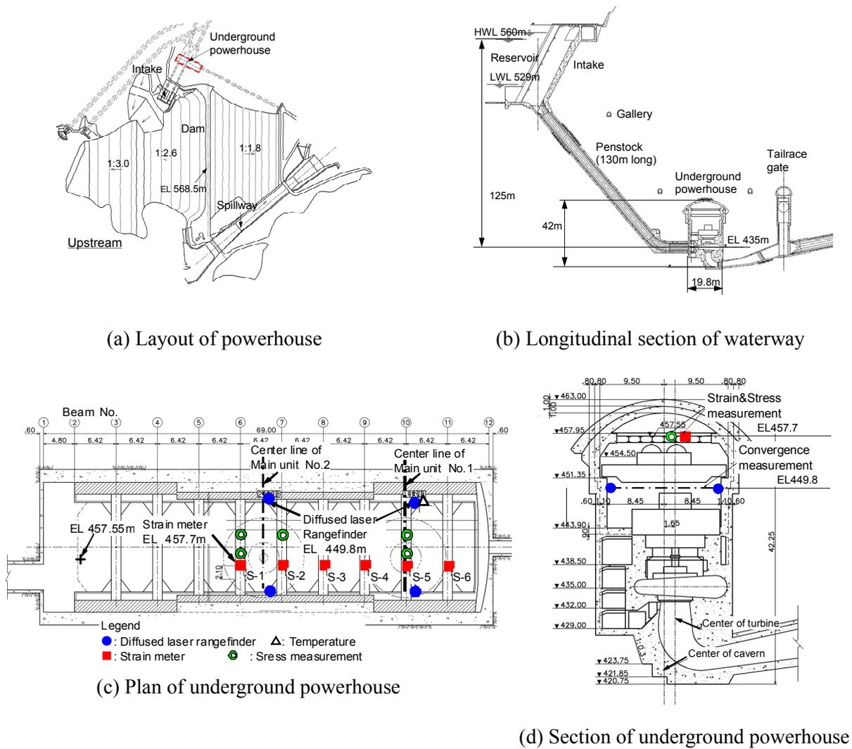
Fig. 1. Underground powerhouse and monitoring arrangement
