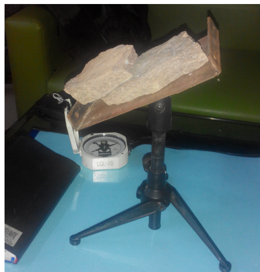
Fig. 7: Experiment determine friction internal angle of intact rock by rock bars
