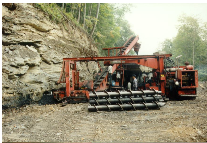
Fig. 6. Auger mining system in Indonesia.
