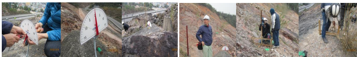
(a) Setting of Mechanical displacement sensor.
