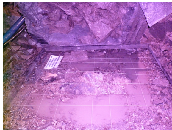
Fig.3b. Inspection of sheared surface after testing
