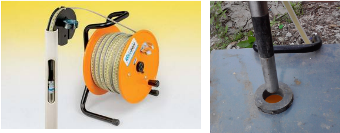
Fig. 6. Schematic structure of monitoring equipment using the magnetic disk
