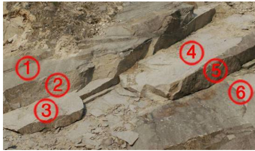
Fig. 11. Discontinuities measured with compass
